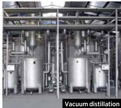
Vacuum distillation evaporation and condensation using inverted cones and centrifugal forces. They are swift and highly efficient in separating constituent elements, which
